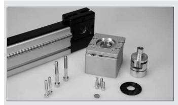
The torques transferred by the clamp connection factor in the maximum mating play for the shaft fits: Shaft k6 / hole H7. Force is transferred from the Coupling to the drive shaft by means of frictional resistance. The shaft and the hole in the hub must be degreased and cleaned to ensure a frictional connec-
