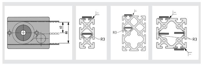
All the cut edges of the profile that face the Timing Belt must be chamfered to prevent irregular running caused by the belt getting snagged or damaged.
