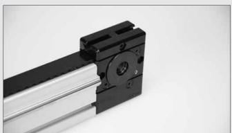
tion for the drive. Fasten the first coupling half to the Reverse Unit, ensuring that the Hexagon Socket Head Cap Screws used are secured against working loose. Clamping screw: T = 23 Nm
