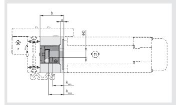
The prepared Coupling fits the drive shaft and transmits drive torque without backlash.
