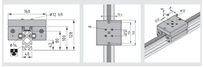
In combination with Profile 8 80x80 as a support profile and Slide LRF 8 D14 200x160:
