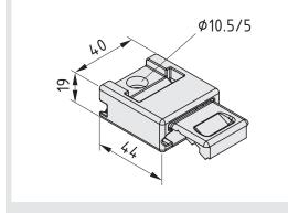
Timing-Belt Tensioner, Tensioning Block 8 R25, 0.0.426.29 [b]
