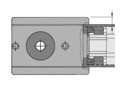
Fastening arrangement of Timing Belt Reverse Unit 8 80 R25 on different profiles depending on the position of the Timing Belt when fed back through.
