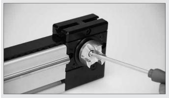
Use Hexagon Socket Head Cap Screws DIN 912 M8x50 (included with the Drive Set, T = 25 Nm) to screw the Coupling Housing of the Drive Set over the entire Coupling through the casing of the Drive Unit.
