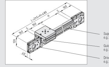
Fundamentally, a Linear Unit converts a rotary motion into a translational motion.
