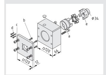
Drive Set ZU 8 80 D55/D34 AP/WP 60 (0.0.672.75) is used solely to connect item drives. The Drive Set is fully prepared for installation on the corresponding Linear Unit. The drive shaft transfers drive torque without backlash.
