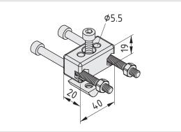
Timing-Belt Tensioner, Fixing Block 8 R25, 0.0.426.30 [a]
