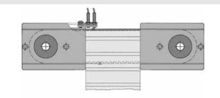
The Proximity-Switch Cams run through Timing-Belt Reverse Unit 8 80 R25. When used on the drive-side Timing-Belt Reverse Unit 8 80 R25, they are particularly useful for simplifying the wiring between Drive Unit, limit switch and motor control unit.
