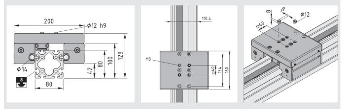
In combination with Profile 8 120x80 as a support profile and Slide LRF 8 D14 200x160:
