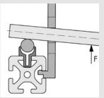
Slot the guide carriage in its preassembled state onto the support profile that you fitted the guiding Shafts to earlier.
