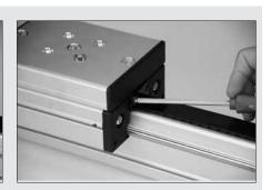
Insert both ends of the Timing Belt into the Tensioning Blocks so that the cavity inside each Tensioning Block is filled then screw securely into place. Fix one Tensioning Block in place under the carriage plate and use the other to tension the Timing Belt with the aid of the long Hexagon Socket Head
