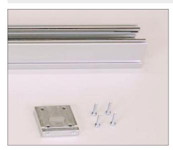
Use four Hexagon Socket Head Cap Screws M5x20 each to screw the two end caps to the right and left ends of the profile. Ensure the end caps are centred on and parallel with the Support Profile then tighten the screw fixings.
