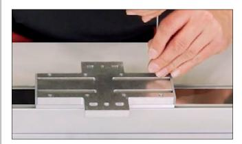
First, use a mallet to fit the Caps X 6 60x12. Centre the transverse carriage plate on the intermediate carriage plate, ensuring both are parallel. Tightening torque  $M_{\tau} = 1.5$  Nm
