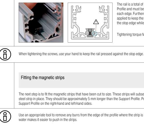
The rail is a total of 20 mm shorter than the Support Profile and must be centred, that is to say 10 mm from each edge. Furthermore, manual pressure must be applied to keep the rail pressed permanently against the stop edge while the screws are being tightened.
