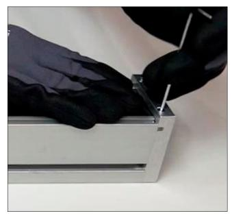
Secure the ends of the steel strip in the end caps. The clamping plate screws need to be loosened by three to four turns for this purpose.
