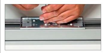
Next, screw the intermediate carriage plate securely onto the body of the carriage using the eight Countersunk Screws M4x10.
