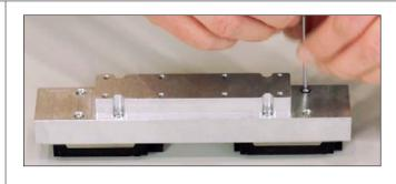
Place the two Bearing Carriages underneath the carriage and also screw these in place.
