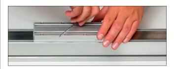
After that, screw on the carriage plate. First, use a mallet to fit the Caps X 6 60x12. Working by hand, centre the carriage plate on the intermediate carriage plate, ensuring both are parallel.
