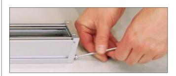
Once everything has been properly fitted and screwed into place, move the carriage over the entire length of the axis byhand, checking the operation and smooth running of the guide.
