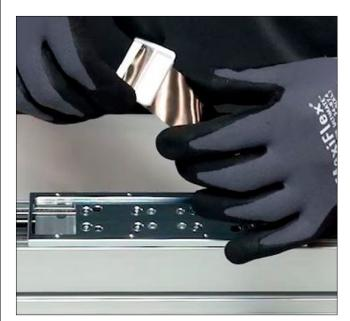
Fit the two guides – correctly aligned – onto the steel strip. The correct alignment of the steel strip guides is important and must be ensured.
