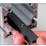
The next step is to fit the linear guide rail. Start by checking the sawn ends of the rail are burrless and rework them if necessary.
