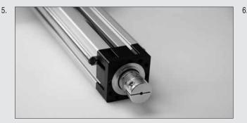
Slot the housing over the fully assembled Coupling and screw it into place using Hexagon Socket Head Cap Screws DIN 912 M8x60 (T = 25 Nm).
